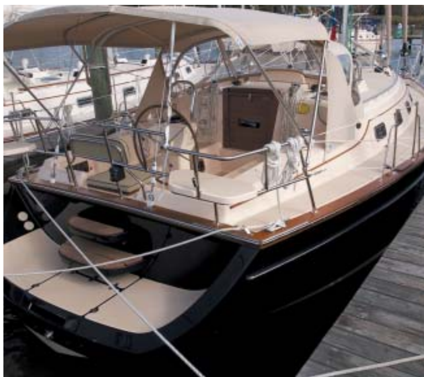
The wheel steering features Whitlock's Premier XL rack-and-pinion direct drive system, a bullet-proof arrangement ideal for long-range cruising.
