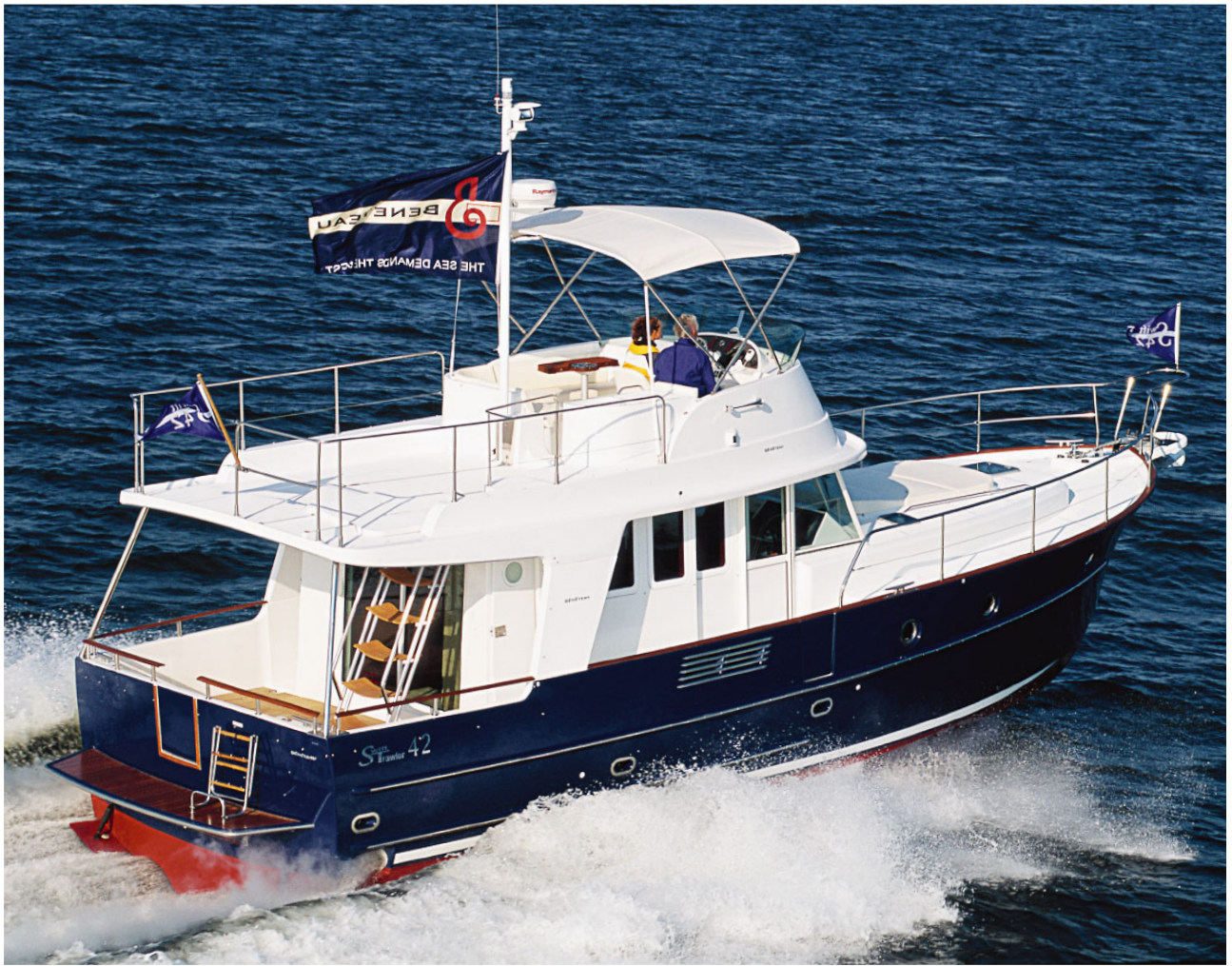
SAFE SHELTER: Stout handrails enclose the foredeck, while high bulwarks and a large overhang protect the sidedecks and cockpit.
